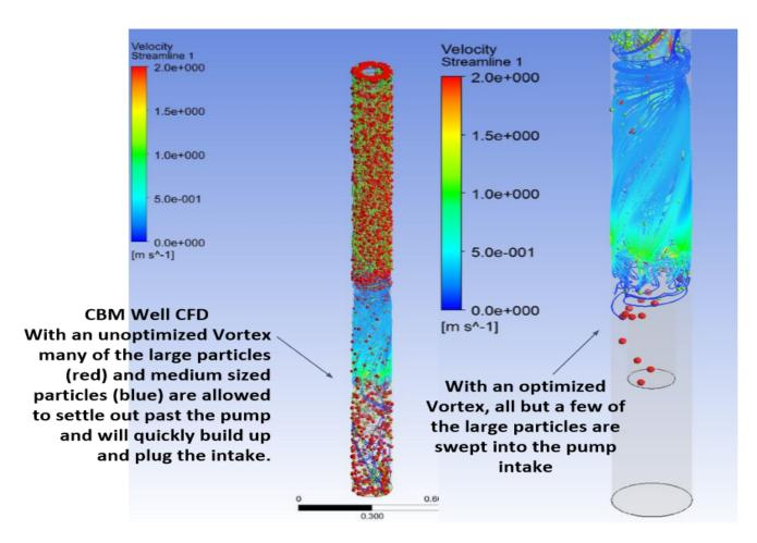
View of the Nozzle velocity profile @ 1,000 psi. This is where the Vortex is optimized for a CBM well.
